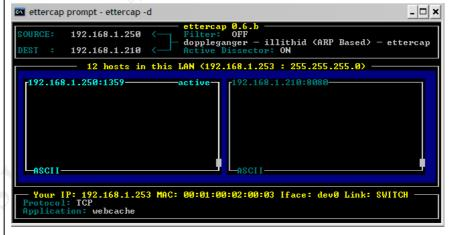
The above screen shows the attempted attack from 192.168.1.253 trying to eavesdrop on a http request from 192.168.1.250 to 192.168.1.210. The 192.168.1.210 is simulating the file server on the storage network and the 192.168.1.250 machine is simulating a client. ARP poisoning was effective but traffic could not be received do to consistent application of the ACLs. The machine making the request suffered from intermittent connectivity as it's ARP cache was poisoned and flushed.
