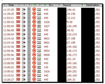
Below snapshot depicts the impact of the Stealth Rule. (NMAP utility is used to scan the IP address of the firewalls.)
