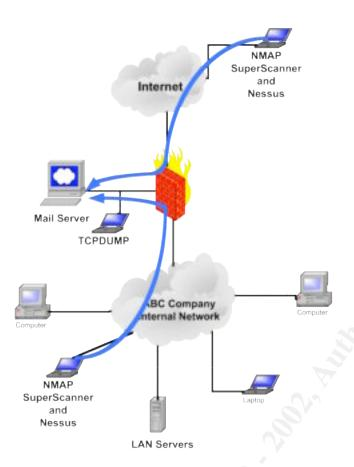
This is an objective test that will positively confirm the access through the firewall that is permitted into the DMZ network. Resources used for this test include training received from SANS, as well as information gathered from <a href="www.cert.org">www.cert.org</a> and www.auditnet.org.
