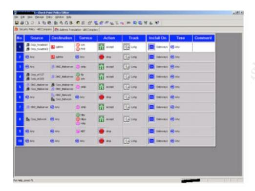
In this configuration the firewall rule permitting email to the Internet (source - DMZ Mailserver, Destination – ANY) has been moved from rule #4 to rule #7. Also a new rule has been inserted as rule #6, blocking all communications to the internal network and the DMZ network.
