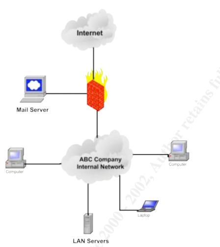
Internet connectivity is through a Checkpoint Firewall version 4.0 running on a Sun SPARCStation system and the Internet connection is through a high speed DBS circuit directly connected to the Ethernet port of the firewall. Connected to a separate port of the firewall in a Demilitarized Zone (DMZ) network is the corporate mail server that is used to send and receive all email messages.
