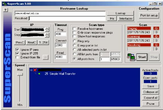
The system running topdump detected only TCP port 25 communications being passed through the firewall:
