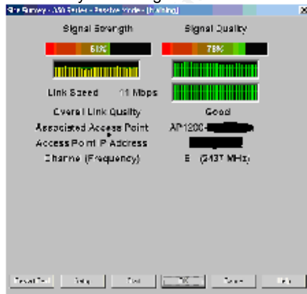
Site survey in training room next to AP
